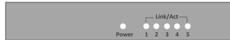
DCGS-2005/DCGS-2005L Switch Tap is implemented the following LED indicators on the front panel:
